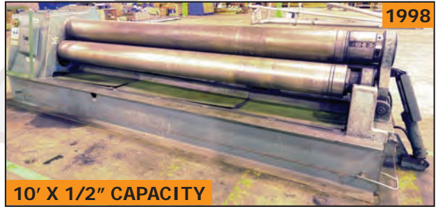
ROUND AB (1998) PS255 hydraulic plate roll
