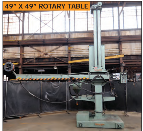
PANDJIRIS cart mounted welding manipulator
