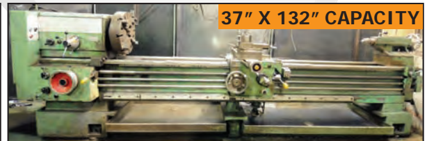
VDF gap bed engine lathe
