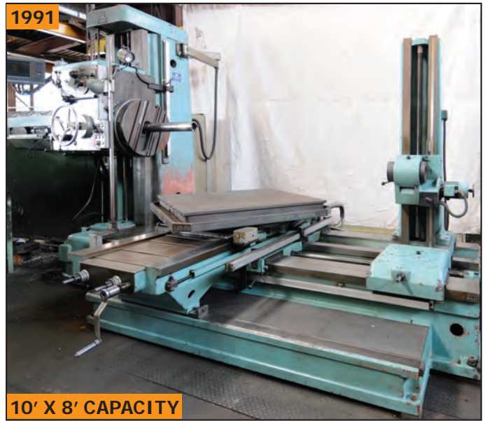
TOS W100A 4" table type horizontal boring mill
