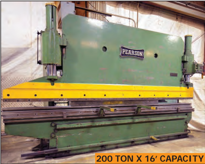
PEARSON 200 ton hydraulic press brake
