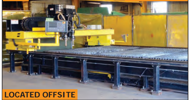
ESAB SABRE SXE 3000 VISPC 3 axis CNC gantry type plasma cutting machine (Professionally dismantled for ease of shipping.)
