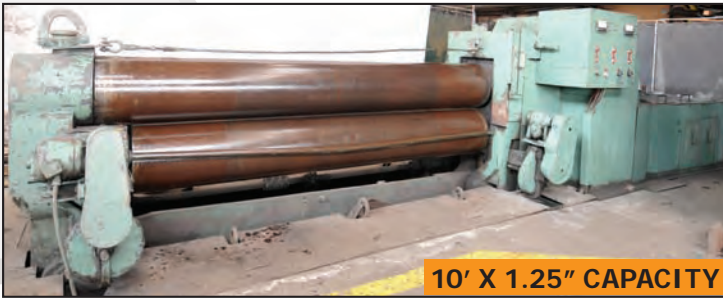
BERTSCH #18 initial pinch hydraulic plate bending rolls
