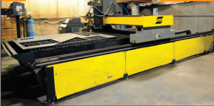
ESAB ACER2 VISPC 3 axis CNC gantry type precision plasma cutting system
