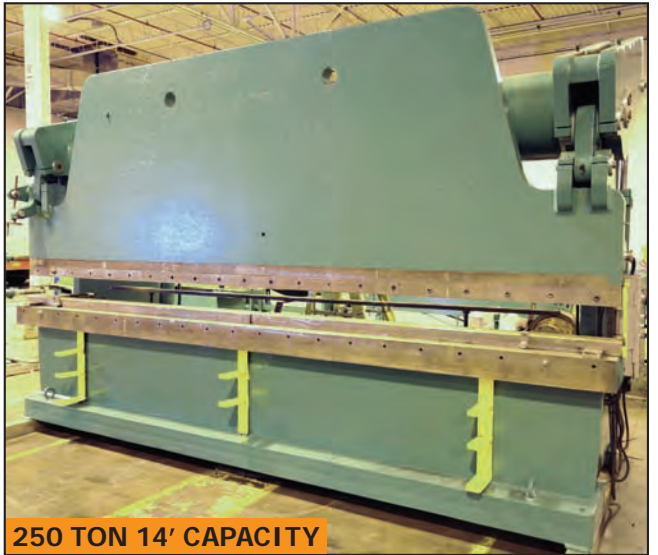
ACCURPRESS 725014 hydraulic press brake
