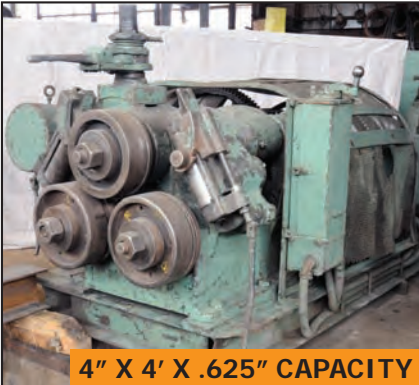
BUFFALO #2 mechanical angle bending rolls
