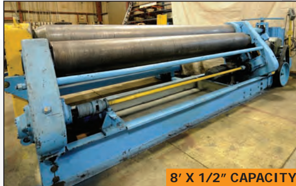
BERTSCH initial pinch power bending rolls
