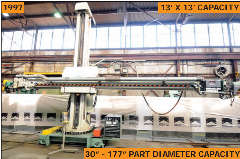
FARROS BLATTER polishing, back gouging and sub arc welding system
