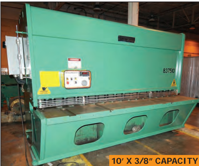
ACCURSHEAR 837510 hydraulic shear
