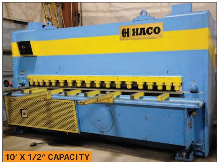
HACO HSL3013 hydraulic shear
