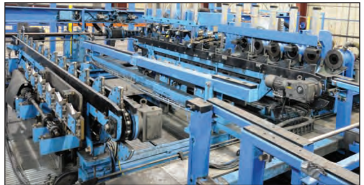
Hydrostatic tube test station and conveyor
