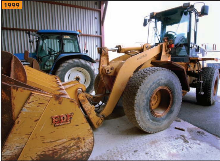
CATERPILLAR 938G front end articulating wheel loader
