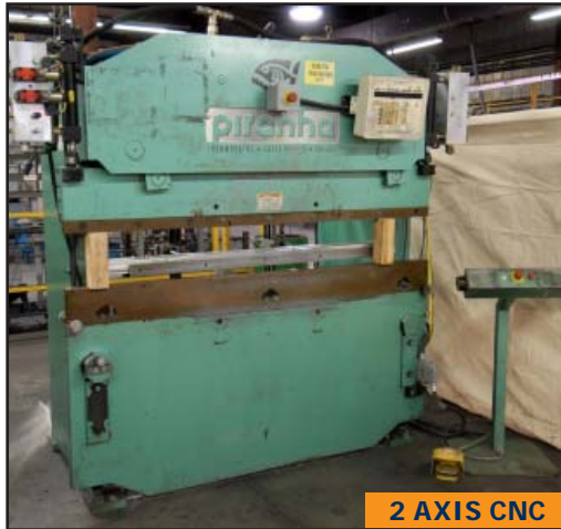
PIRANHA 3506 35 ton hydraulic press brake
