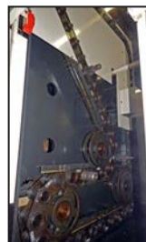
View of 60 station ATC
