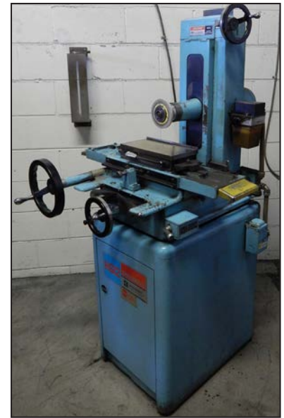
BOYER SCHULTZ CHALLENGER H612 hydraulic surface grinder
