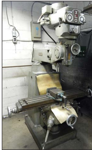
EXCELLO 602 vertical milling machine
