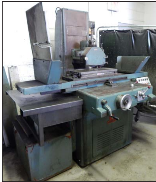
NYBERG & WESTERBERG AB TYPE 650-350 hydraulic surface grinder
