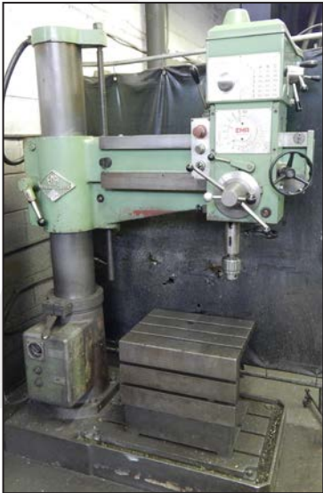
EMA radial arm drill
