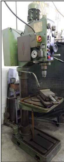
IBARMA gear head drill
