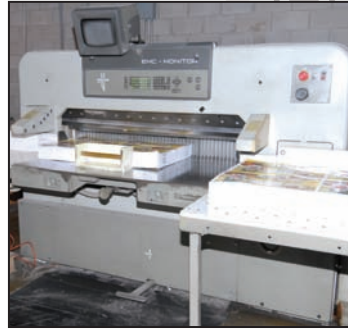
POLAR MOHR 137 EMC-MON hydraulic paper guillotine
