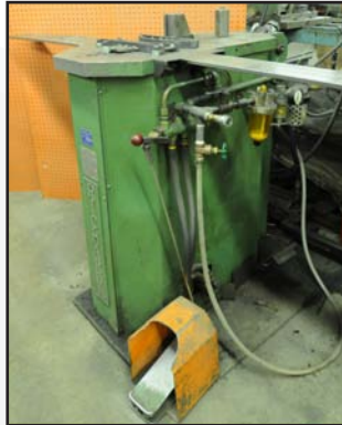
RICHARDS MULTIFORM hydraulic bender
